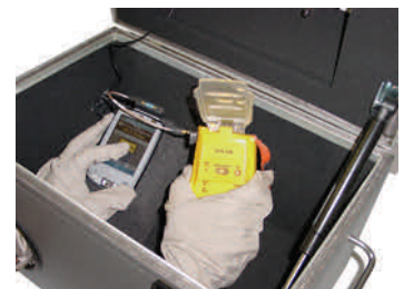
Screened Testing Box – Faraday Cage
