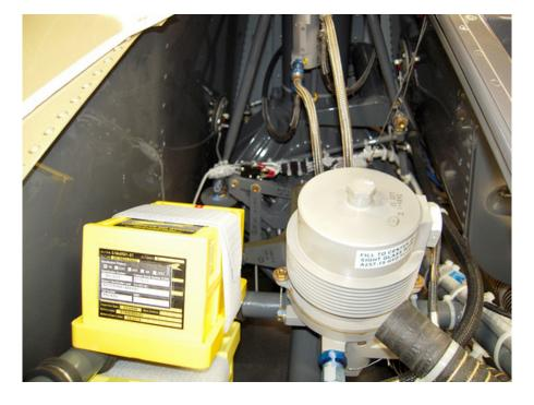
The main mast to the rotor can crush the ELT especially if it is a R22 or R44
