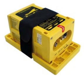
Example of INTEGRA ELT installed on a Universal Mounting Bracket
