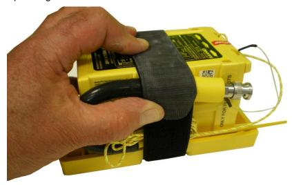
3. Firmly adjust and tighten the retaining strap.
