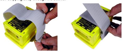
Ensure the buckle is correctly positioned (indifferently on right or left side of ELT)
