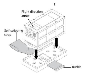
Place the antenna and tether onto the mounting bracket, on the opposite side of the buckle, fold the antenna, BNC connector to the top, and slide the antenna and the tether between the strap and the ELT. Keep them maintained by the strap while sliding the selfstripping strap through the buckle.
