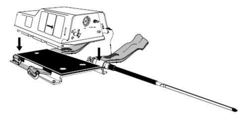
2. Fold the antenna and slide it though the elastic loops of the hook and loop fasteners
